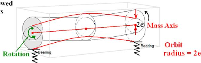
(produces very high bearing forces if bearing clearances are insufficient to allow the increased displacement)
