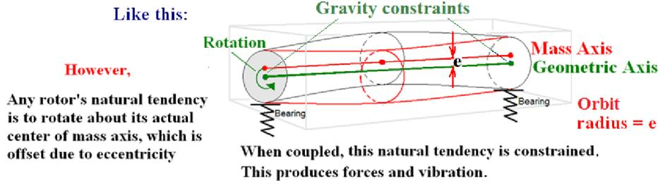
Natural tendency of a bowed rotor is to rotate about its center of mass axis.
