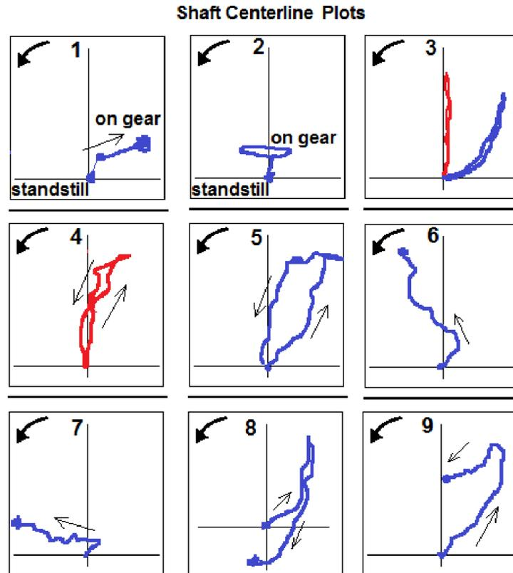
**Fig.2.** Representation of commonly seen shaft centerline plots, including common faults. The two paths in Plot 3 represent the "ideal" for tilting-pad and elliptical bearings, respectively.
