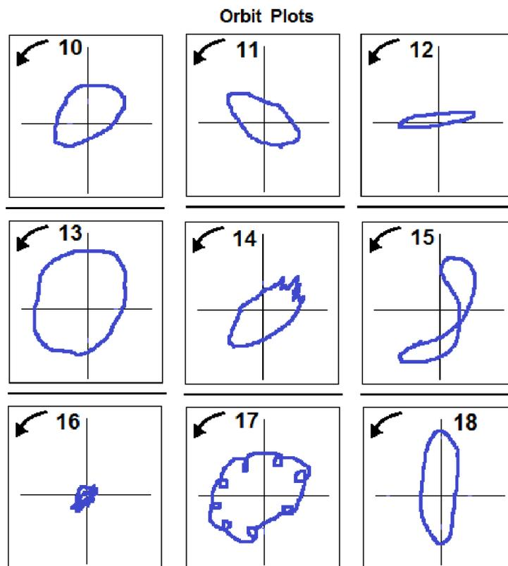
**Fig.4.** Representation of commonly seen shaft orbit plots, including common faults.
