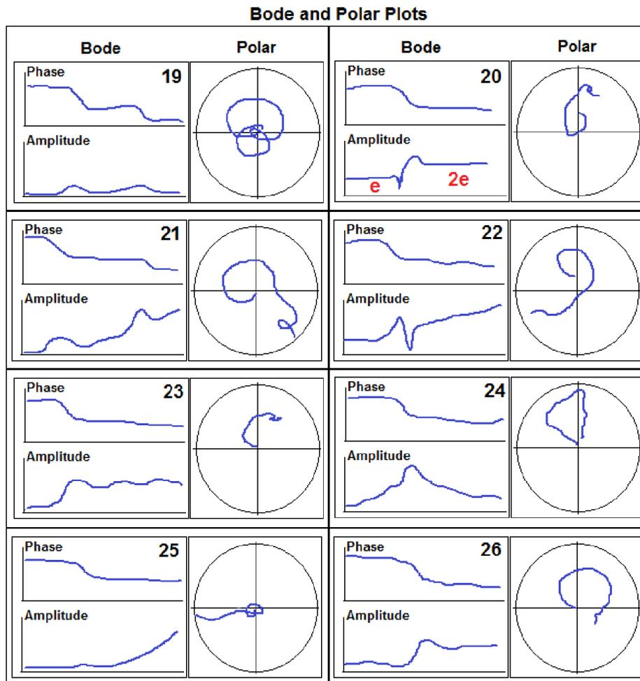
**Fig.3.** A representation of commonly seen Bode and Polar plots indicative of mass eccentricity. Plot 19 represents the idealized Bode and polar plot for a rotor with minimal eccentricity.
