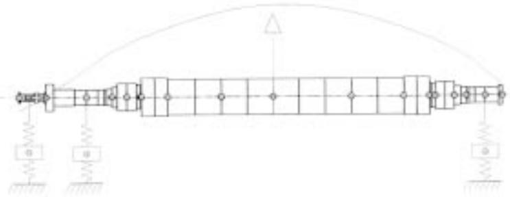
**Figure 19C: Rotor Calculated 2nd Mode**
