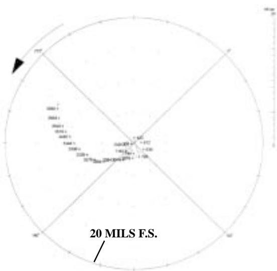
**Figure 4: Start Up with First Trial Run- 760 gr. @ 180° st. (GENRR)**
