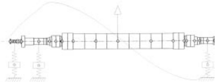
**Figure 19D: Rotor Calculated Undamped 2nd Mode**
