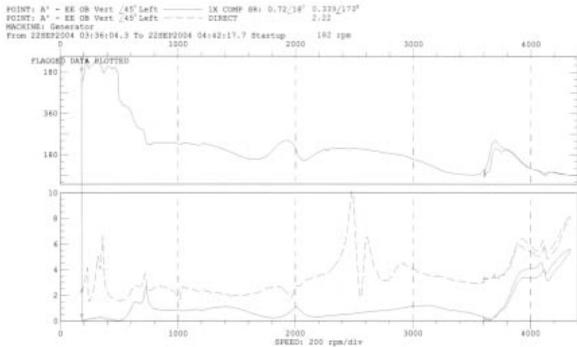
**Figure 19: Third Critical– Not Fully Balanced (GEN-REAR)**
