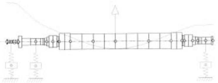
**Figure 19E: Rotor Calculated Damped Deflection Shape at 3600 RPM**
