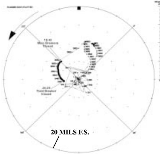
Figure 10: "Thermal Vector" Change During Field Excitation (GENRR)
