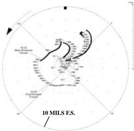
Figure 12: "Thermal Vector" Wandering with Load Increasing (GENFR)
