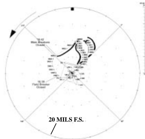
Figure 13: "Thermal Vector" Wandering with Load Increase (GENRR)
